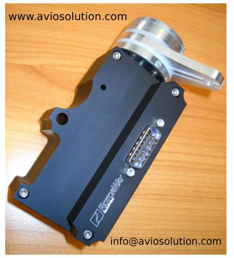
By reading the Fadec Canbus it's able to know the engine load and to optimize the engine control also with abrupt maneuvers.
